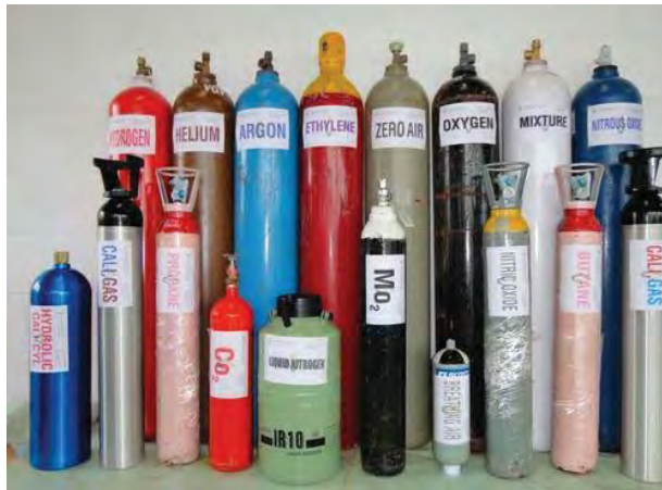
Figure: Color coded Gas Cylinders
