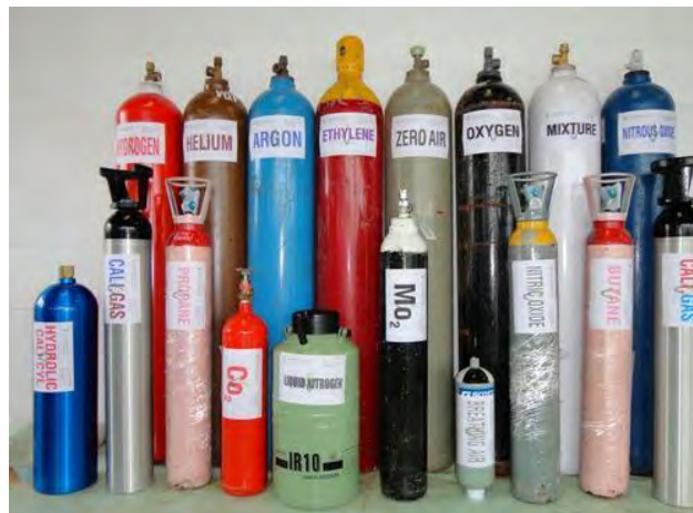
Figure: Color coded Gas Cylinders
